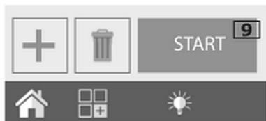
The appliance will start operating in pre-heat mode if this has been previously selected. Otherwise, it moves directly to the thermal processing mode.
