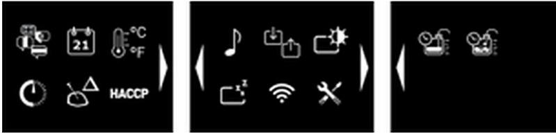
Using the push rotary controller, you can navigate through the three screens and select the settings.
