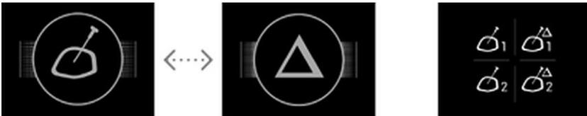
The appliance is equipped with a thermal core probe in the thermal processing chamber. In addition, two additional external thermal core probes can be connected to the appliance.
